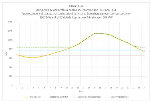
Figure 3.3-90 Western LA Basin LCR Sub-area 2025 Annual Load Profile with Estimated Transmission Load Serving Capability Only (with Laguna Bell – Mesa 230kV#1 line upgrade)
