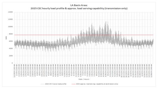
Figure 3.3-89 Western LA Basin LCR Sub-area 2025 Load Shape and Estimated Maximum Energy Storage Capacity and Energy Based on Charging Capability Under Critical Contingency (without Laguna Bell – Mesa #1 230kV line upgrade)
