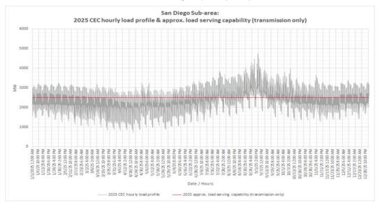
Figure 3.3-102 San Diego LCR Sub-area 2025 Load Shape and Estimated Maximum Energy Storage Capacity and Energy Based on Charging Capability Under Critical Contingency
