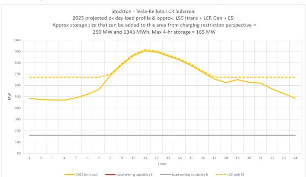
Figure 3.3-29 Tesla-Bellota LCR Sub-area 2025 Peak Day Forecast Profiles
