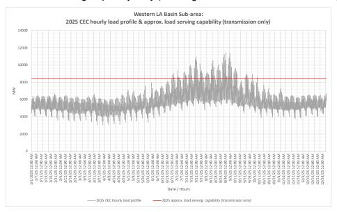
Figure 3.3-91 Western LA Basin LCR Sub-area 2025 Load Shape and Estimated Maximum Energy Storage Capacity and Energy Based on Charging Capability Under Critical Contingency (with Laguna Bell – Mesa #1 230kV line upgrade)
