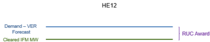
Figure 1: Procurement of additional capacity is needed to address the forecast difference between IFM and the net load forecast.
