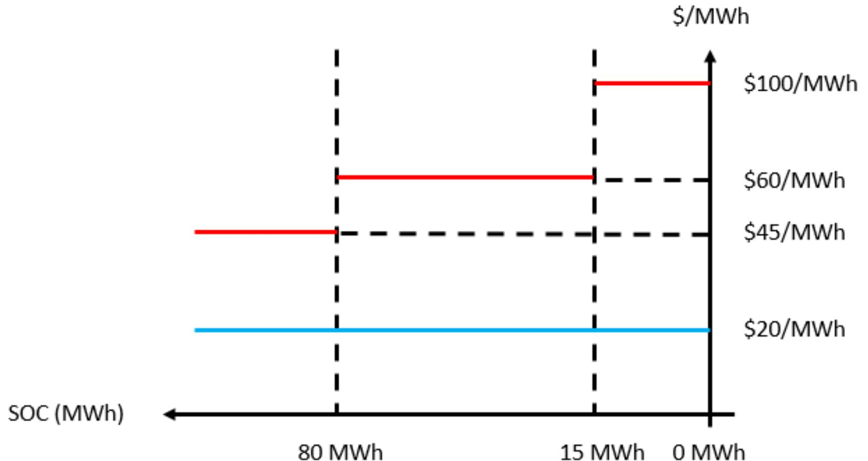
The storage resource will discharge when prices are above \$60/MWh, at medium states of charge
