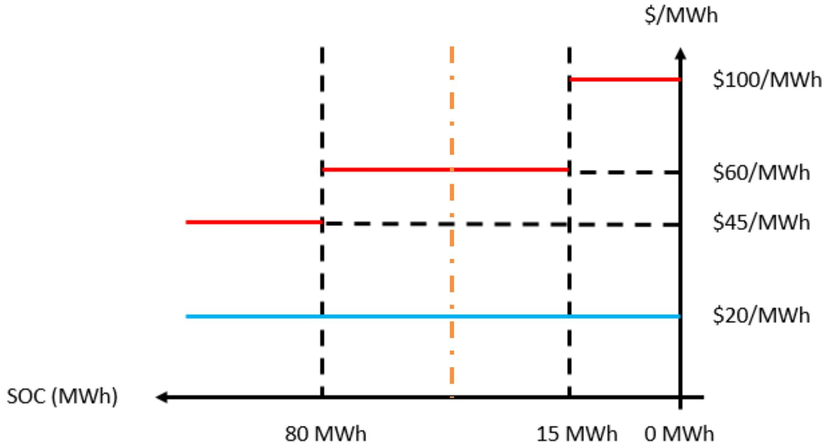
The storage resource will discharge when prices are above \$100/MWh, at low states of charge
