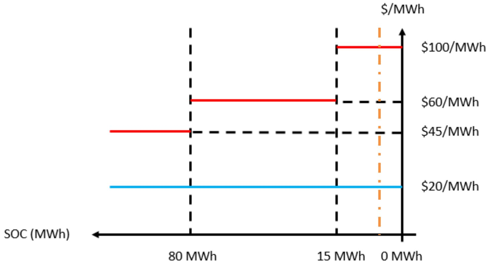
The storage resource will discharge when prices are above \$45/MWh, at high states of charge
