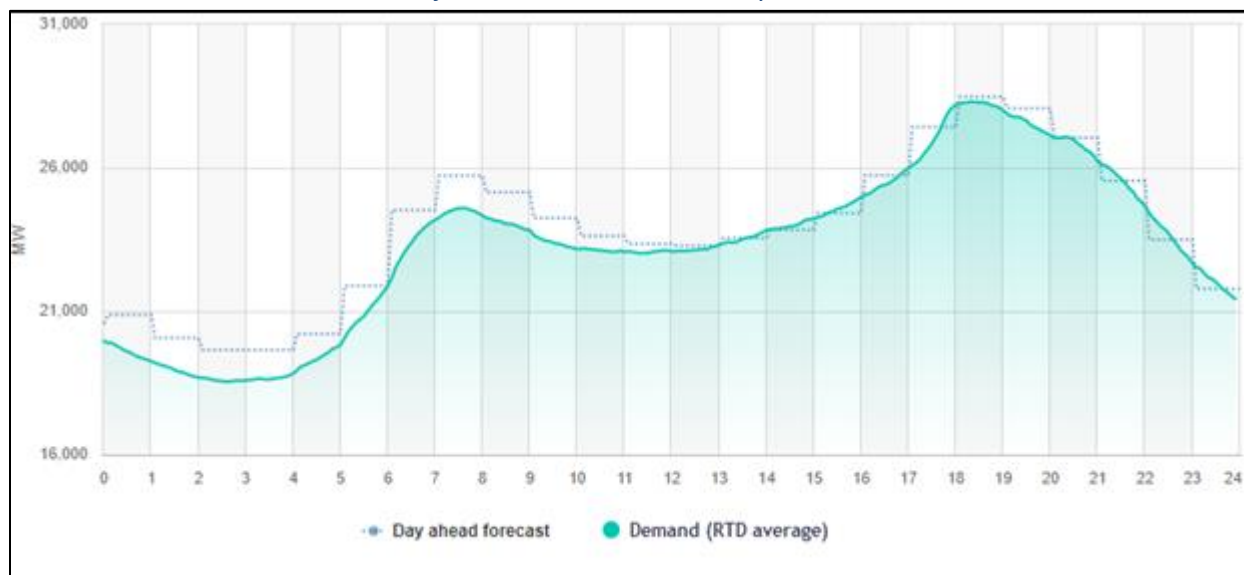
Figure 1: Day-Ahead Market hourly procurement in comparison to real-time demand curve. California ISO Trade Date February 5, 2018.
